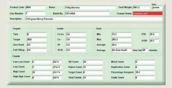
The checkweigher screen shows the product being monitored, together with all of the count and statistical data.
